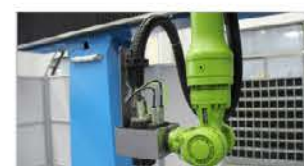
Anti-collision protection system for cutting head 切割头防撞保护系统
